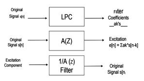
Figure 2. Speech analysis and synthesis process.
