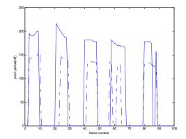
Figure 4. Pitch of speech signal, (-) old pitch of the signal, (-.-.) new pitch of the signal.
