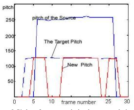
Figure 8. Pitches of source morphed and target speech signal.
