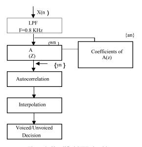
Figure 3. Simplified SIFT algorithm.
