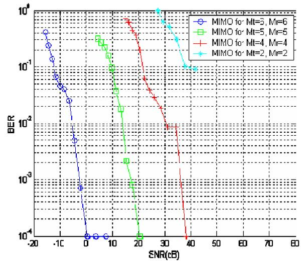
Figure 6. LMS-MIMO-MCCDMA performance in the AWGN with multi-path Rayleigh fading channel (with the variation of the transmitter and receiver antenna elements).
