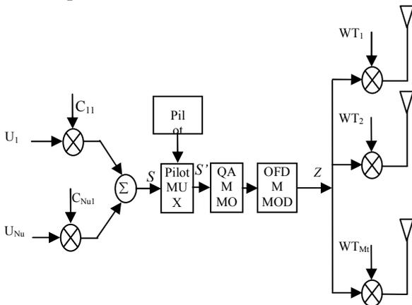
Figure 1. LMS-MIMO-CCDMA transmitter.
