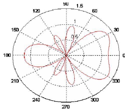
Figure 5. Beampattern response for two interferences (at  $135^\circ$  and  $300^\circ$ ) and desired signal at  $45^\circ$ .
