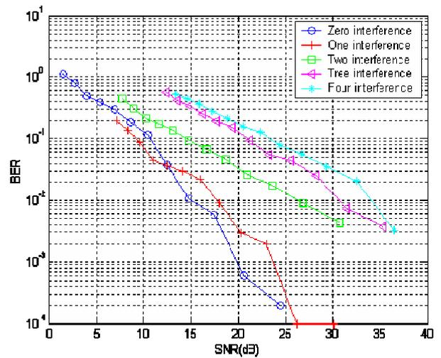
Figure 7. LMS-MIMO-MCCDMA performance in the AWGN with multi-path Rayleigh fading channel (with increase number of interferences).
