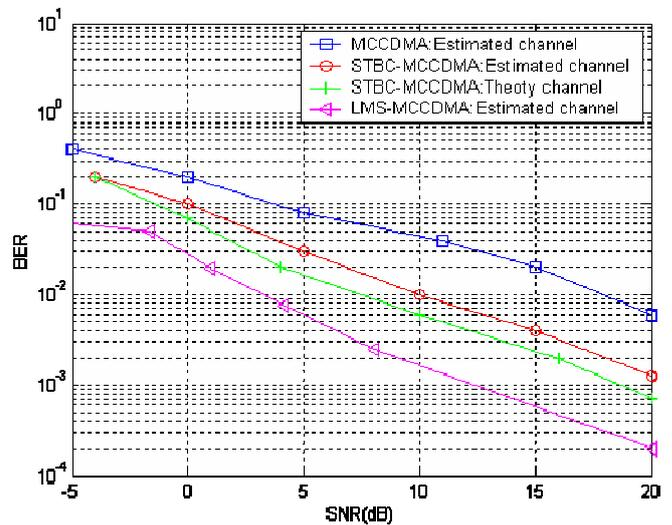
Figure 4. Performance comparison between LMS-MIMO-MCCDMA system and STBC-MIMO-MCCDMA system (for MIMO  $M_t=M_r=3$ ).
