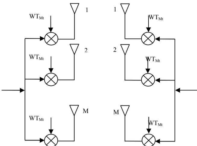
Figure 3. A MIMO system model.
