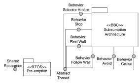
Figure 6. Pattern-level with control interface diagram for intelligence behavior.
