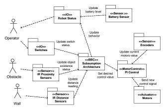
Figure 3. Pattern-level diagram for the AMR software.
