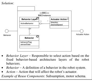
Figure 1. Behavior-based control pattern catalogue.
