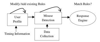
Figure 2. Signature based intrusion detection system.
