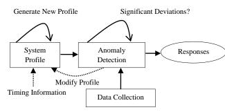
Figure 1. Anomaly based Intrusion detection system.
