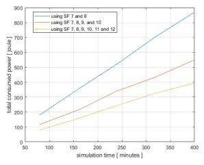
Figure 5. The total consumed energy in the new algorithm at different SF values.
