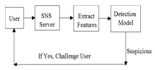
Figure 4. Principal flow of the fraud detection scheme.
