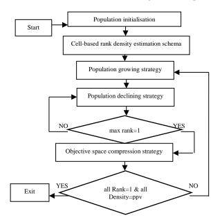
Figure 2. DMOEA algorithm flowchart [10].
