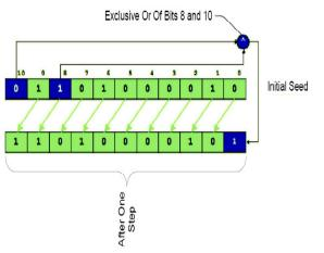
Figure 2. A model LFSR to be used in BGS cipher.
