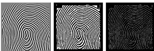
(a) Enhanced image. (b) Binarization image. (c) Thinned image.
