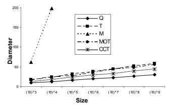
Figure 13. Diameter comparison for interconnection networks of different sizes.
