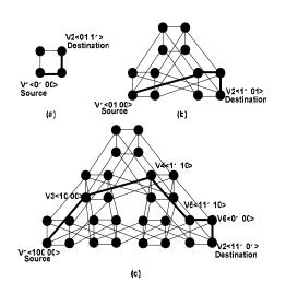
Figure 8. The maximum distance (diameter) between two nodes (v1, v2) in *CCT*: (a) *CCT* (0, 2); (b) *CCT*(1, 2); (c) *CCT*(2, 2).
