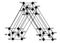
Figure 4. Vertical parent-child links for CCT (1, 3) for nodes 110.
