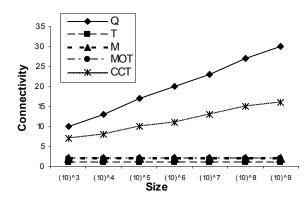
Figure 16. Connectivity comparison for interconnection networks of different sizes.
