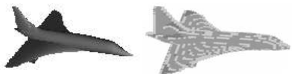
Figure 2. The voxel representation for a model of an airplane from the PSB database.
