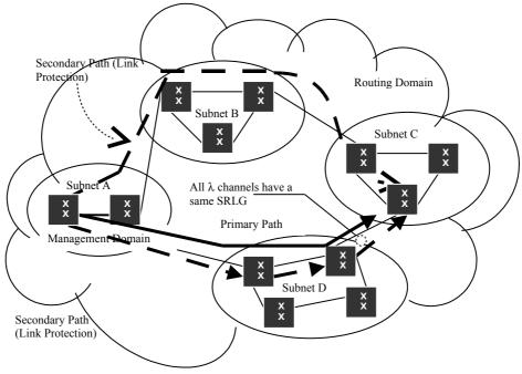
Figure 4. Light path protection vs. link protection.
