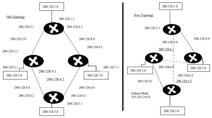
Figure 1. IP layer addressing in an IP over reconfigurable WDM network.
