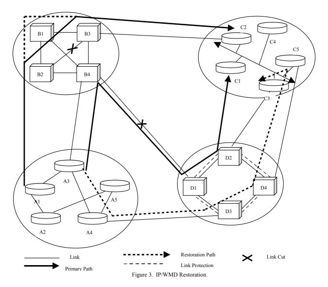
In principle, dynamic restoration can be applied to sub-wavelength channels or very fine-granularity virtual channels, but that level of restoration usually generates a significant amount of control traffic and therefore hinders its 'real time' performance and subsequently scalability. Path protection/ restoration has three variants:
