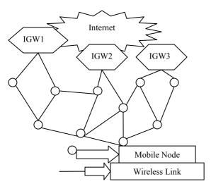
Figure 1. Mobile ad hoc network connectivity with Internet.
