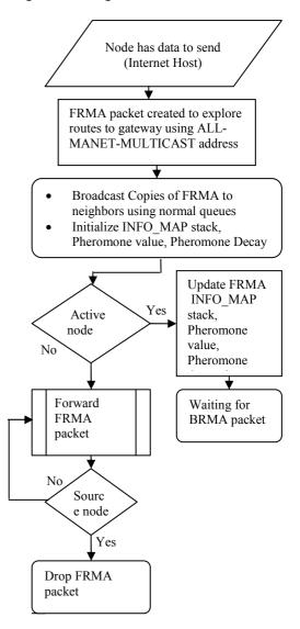
Figure 2. Process in mobile source node using AODV ALMA.
