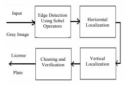
Figure 2. Plate extraction module.
