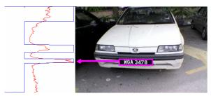
Figure 5. Horizontal projection of the edge image.
