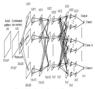
Figure 6. Implemented neocognitron structure.
