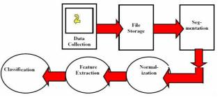
Figure 4. Assyrian machine printed character recognition system processing steps.
