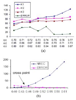
Figure 8. Experiment1: Training for 100 images, varying activation thresholds, (a) network structure size (K1, K2, K3) and ERROR, varying the training threshold  $\theta_1$ ,  $\theta_2$ , and  $\theta_3$ , (b) recognition response NREC (non-classification) and ERROR (misclassification) at the stable region, varying the recognition threshold  $\theta_2$ .
