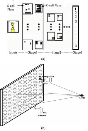
Figure 5. (a) The basic structure of the neocognitron of letter alap in Assyerian character, (b) General structure of S and C cell planes.
