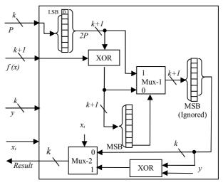
Figure 2. GF(2k) modulo reduction hardware.
