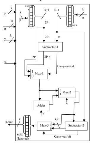
Figure 1. *GF(p)* modulo reduction hardware.
