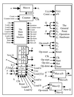
Figure 8. Proposed ECC coprocessor hardware.
