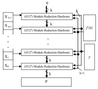
Figure 4. Unfolded  $GF(2^k)$  parallel multiplier.
