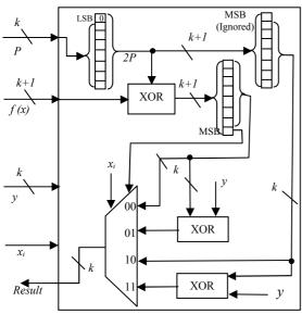
Figure 3. Modified  $GF(2^k)$  modulo reduction hardware.
