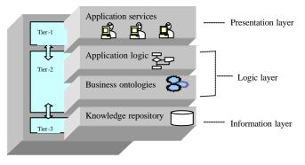
Figure 6. A layered architecture of LiSER.
