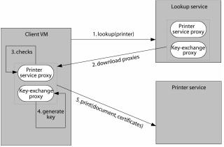
Figure 11. Accessing a Jini service with self-signed certificates (Andersoon's model).
