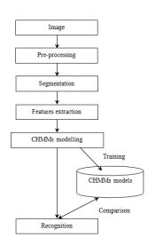
Figure 2. Architecture of continuous hidden markov models.
