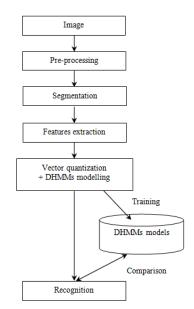
Figure 1. Architecture of discrete hidden markov models.
