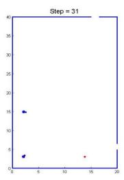
Figure 3. The initialization of two agents and their selection to the nearest exit (the lower exit).
