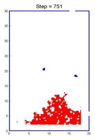
Figure 4. The agent far away from the lower exit made a decision at the tactical level directing his movement towards the upper exit.
