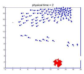
Figure 13. The evacuation of 100 agents distributed randomly in the upper region of the hall (the extended model).
