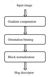
Figure 7. The process of HOG descriptor acquisition of Arabic square root symbol.
