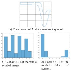
Figure 8. The global and local chain code histogram descriptor: (a), (b) and (c).
