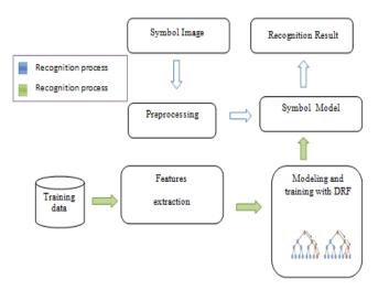
Figure 5. System architecture for the recognition of isolated mathematical symbol.
