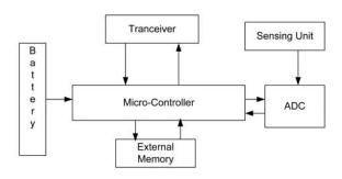
Figure 1. Sensor Node Architecture.
