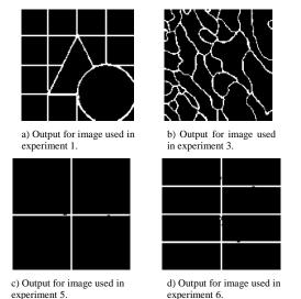
Figure 8. Edge detection output of the test images with noise
