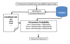
Figure 2. The schematic design of RWSC algorithm.
