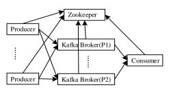
Figure 3. Construction of data buffer.
