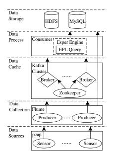
Figure 1. Collaborative threat detection architecture.
