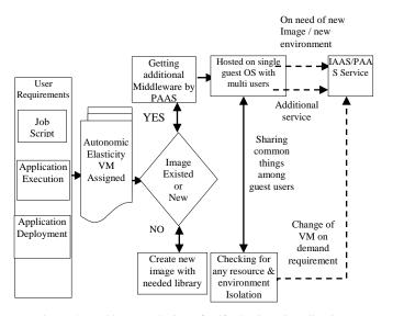
Figure 4. Architecture design of self adaptive virtualization.
