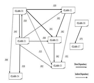
Figure 3. Weighted coupling graph of all possible coupling of package PKG.
